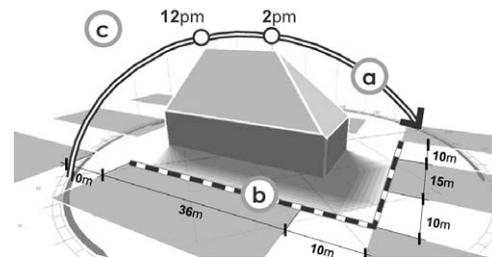
Fig. 2. Parameters used to generate a solar envelope
