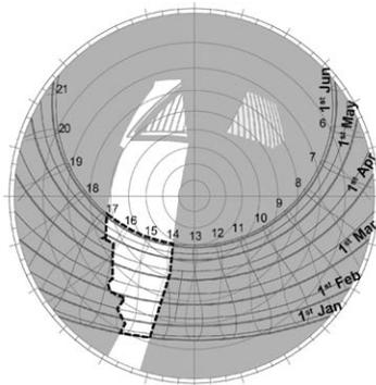
Fig. 7 : Stereographic projection of annual solar access to Level 1 variable occupancy unit – dotted line indicates hours of solar access
