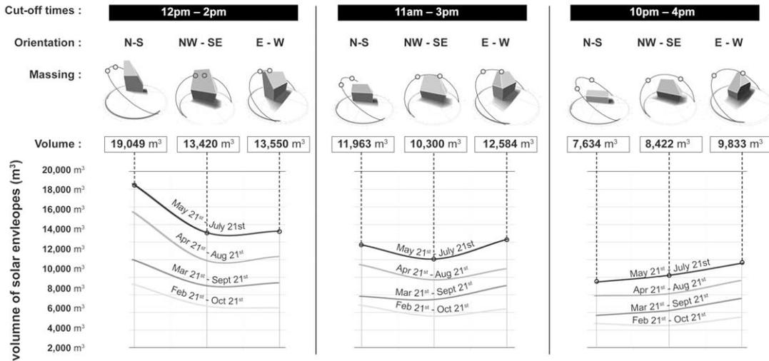
Fig. 3: Variation of volume of solar envelope for different orientations and cut-off times. Solar envelopes from the May 21<sup>st</sup> – July 21<sup>st</sup> series are shown
