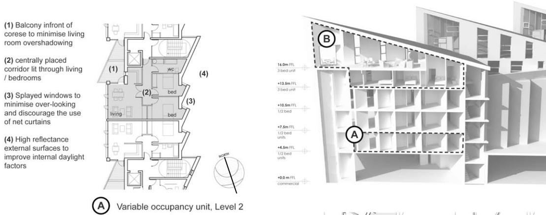
Fig 6: Block B: Apartment plans and perspective section
