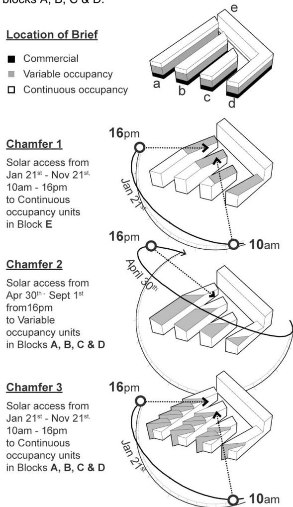
Fig. 5 Chamfers used to provide solar access to units according to occupancy patterns
