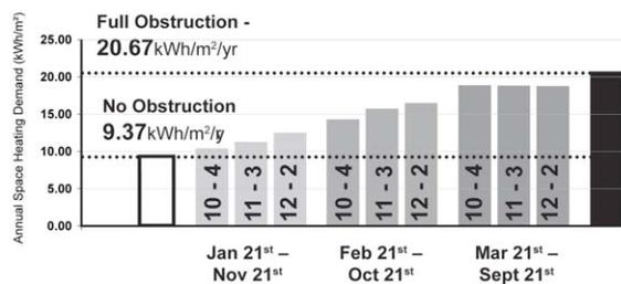
Fig. 4: Annual space heating demand with varying cut-off times for solar access
