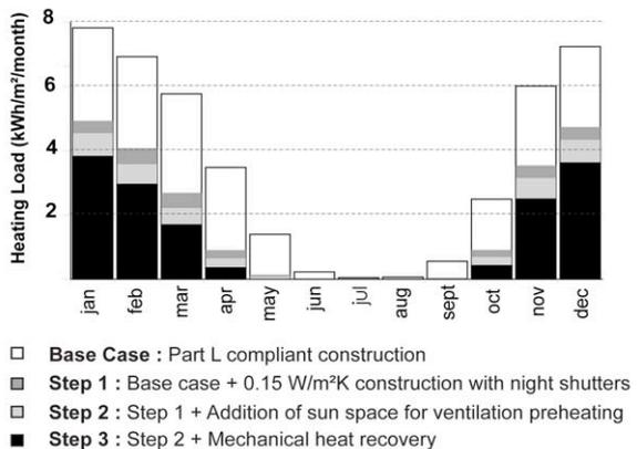
Fig 10: Monthly space heating demand for top floor continuous occupancy unit showing iterative improvements to reduce the space heating demand to within PassivHaus standards
