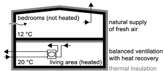
Fig 6. Ventilation concept with two compartments
