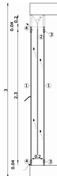
Fig 1. DSF section view: 1) 6 mm glass layer; 2) solar protection (blade width  $W=0.025$  m); 3) aluminium frame; 4) ventilation openings.
